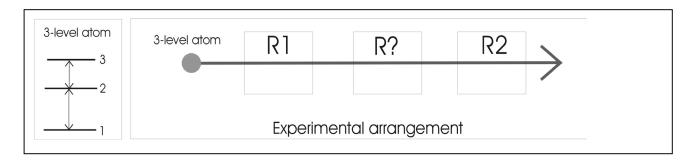
Consider a three-level atom which passes through two pulsed oscillating fields (labeled R1 and R2) of which the frequency is resonant with the transition between state  $|1\rangle$  and  $|2\rangle$ . Between R1 and R2 the atom passes through an area R?, which might or might not contain an oscillating field of which the frequency is resonant with the transition between state  $|2\rangle$  and  $|3\rangle$ . When the R? field is present its pulse length corresponds to a  $2\pi$  pulse.
